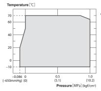
Please use within the operation range of maximum operation pressure and maximum service temperature.
